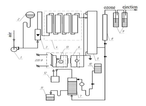
**Figure 1** The scheme of plants for ozonation: 1 - compressor; 2 - monostat; 3 - flowmeter; 4 - the block of air drying; 5 - the ozone generator; 6 - step-up transformer; 7 - bubble column; 8 - spectrophotometer; 9 - Drexel glass with a solution of KI; 10 - a container of cleaning solution; 11- the tank with clean solution; 12 - drip tray; 13 - the linear autotransformer.
