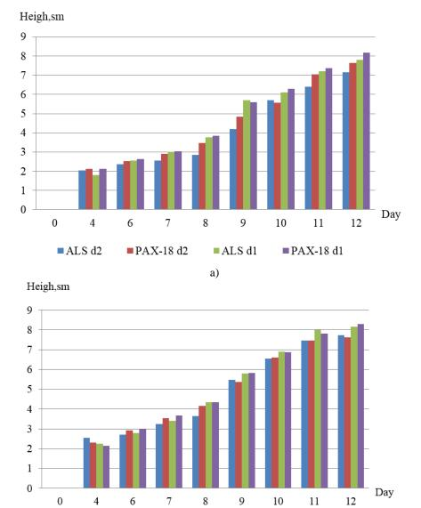
experiments were used. Fig. 3 (a, b) shows the results of determining the influence of aluminum coagulant's with different (OH/Al) ratios on PAP availability of coagulated sludge.
